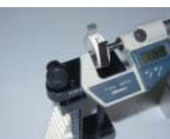
The Micro Checker can be used in either horizontal or vertical orientation, as shown in the picture left.
